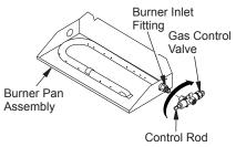
Figure 8 - Installing Gas Control Valve
